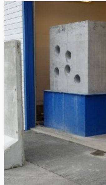
Testing of the new RSS included drilling directional holes through concrete. A total of 10 concrete drilling tests were performed with Prototype C, with a different directional response tested for each hole. The concrete mix was designed with a compressive strength similar to formations in which the RSS would be expected to drill.
