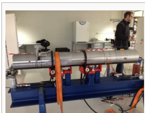
2TD Drilling and a major operator undertook a comprehensive design-test-verification process, including four prototypes, to develop the OrientXpress RSS, which will begin field trials in the US this year. Prototype B verified that the steering head could deliver adequate forces to create a steering response and survive the loads in a downhole drilling environment. This model led to the development of the first full-system prototype.
